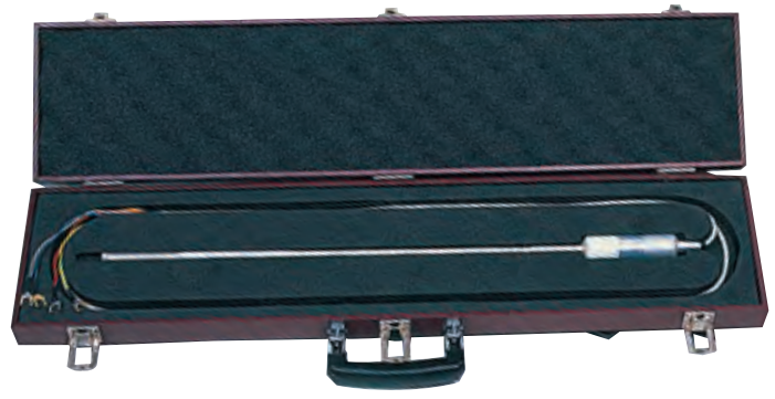
Super Stable Standard Platinum Resistance Thermometer
